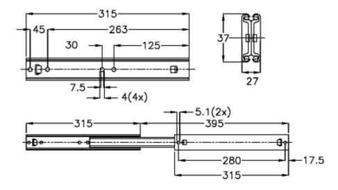
Load capacity bottom mounted = 25 Load capacity side mounted = 50
